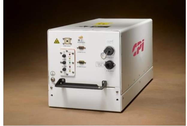
CPI 650 W Ka-band TWTA, provides up to 304 or 290 watts of linear power at the flange, depending on configuration.
